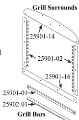
Complete Factory Grill 2. Carefully remove the complete factory grill from hood and remove the Freightliner logo (see diagram to the left). Retain
